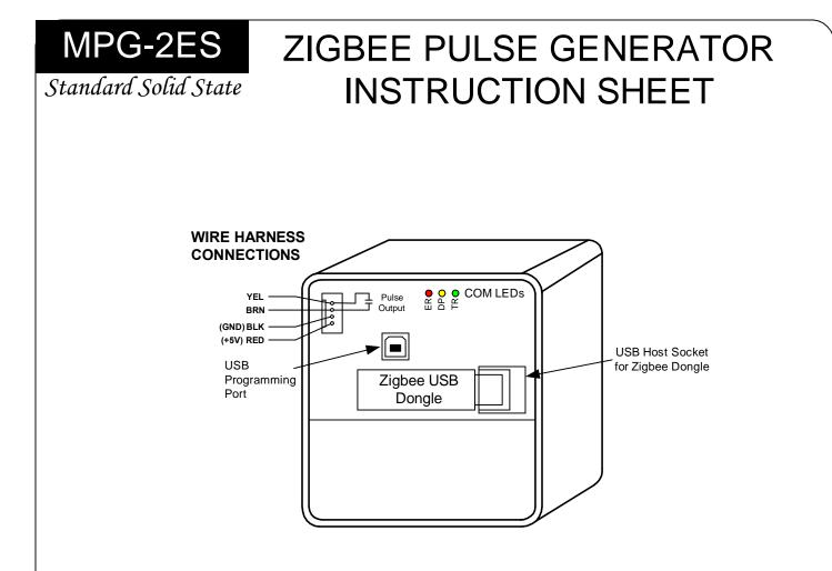
**<u>GENERAL</u>** - The MPG-2ES is a scaled-down, specific purpose version of the MPG-1C and MPG-2 that allows cost reduction when only basic features and one K-Y output are needed.
